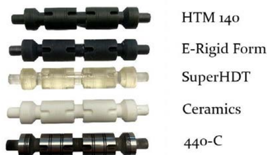
Figure 1: 3D printed polymeric and ceramic spools compared to conventional spool made from 440-C.
