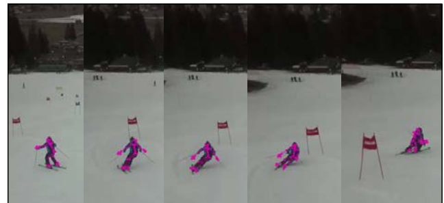
Figure 4: Sequence of frames with skeleton tracking. Skeleton tracking has potential for future drone assisted MoCap measurements.
