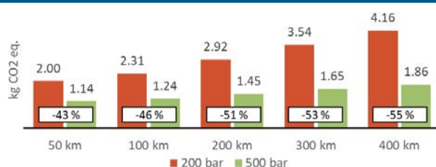
Figure 3: Total GHG emissions of the hydrogen supply chain for different transport distances in Slovenia.
