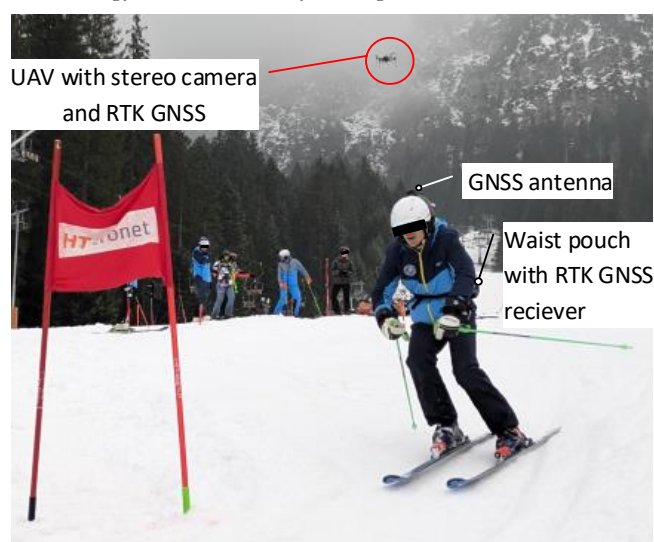
Figure 1: Skiing kinematic measurements with two independent systems.
